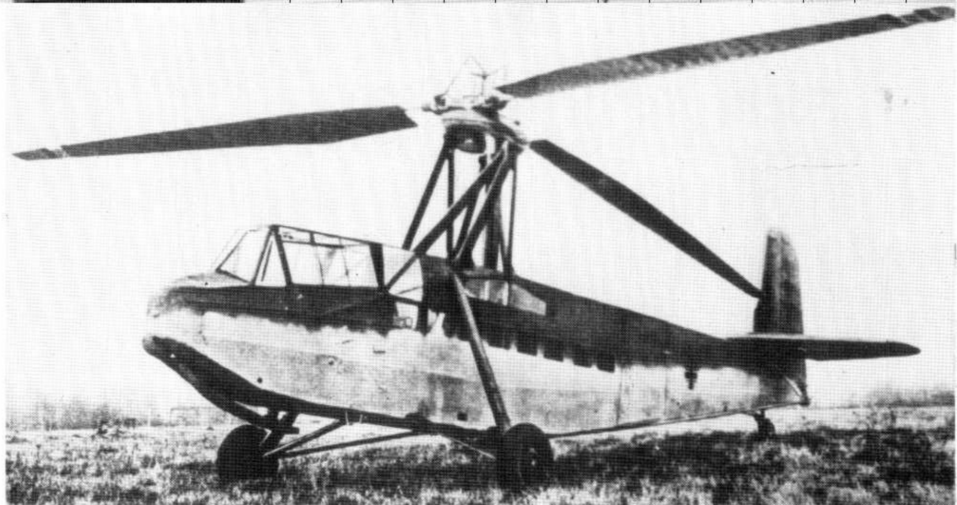
The Fa 225 towed helicopter, with the fuselage of a DFS 230 and the rotor of an Fa 223.
