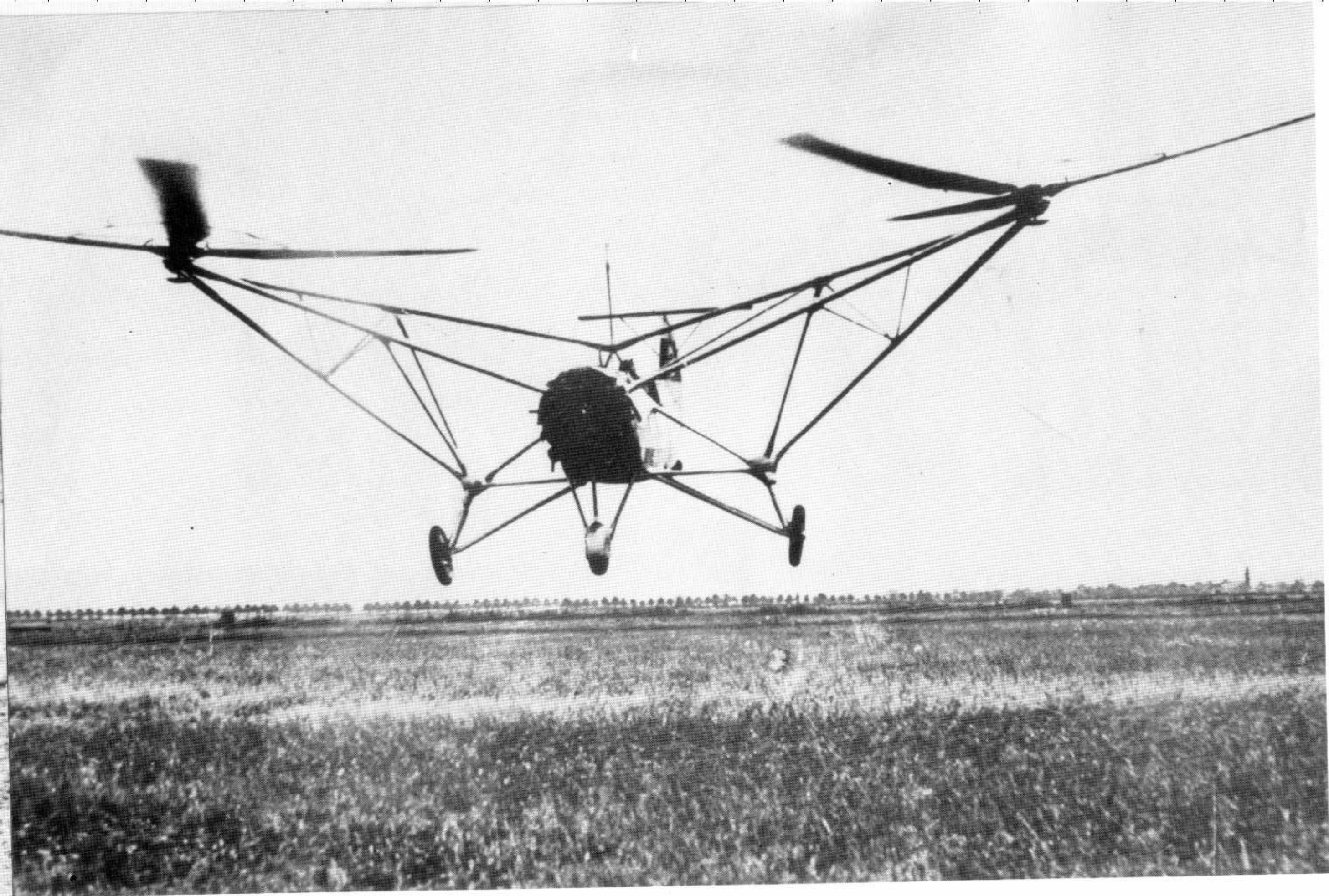
Fw 61 V 1 and V 2 were the first helicopters that could really take off and land vertically. Factory pilots Rohlf, Dipl.Ing. Francke from Rechlin, and Hanna Reitsch took part in the record flights.
