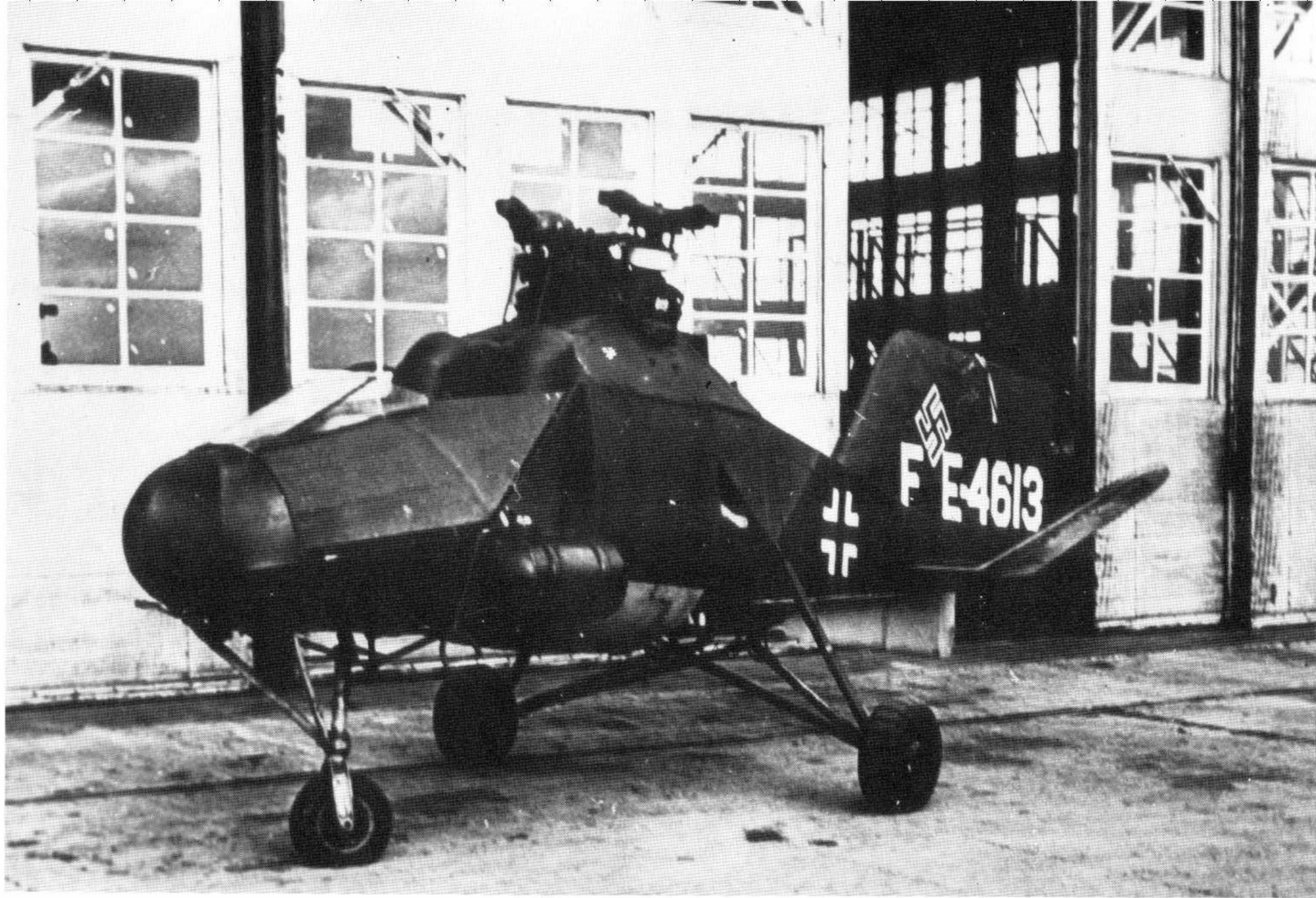
FE 4613 (FE = Foreign Equipment) was the Fl 282 V 23, factory number A-019. The rotor blades have been removed for transportation.
