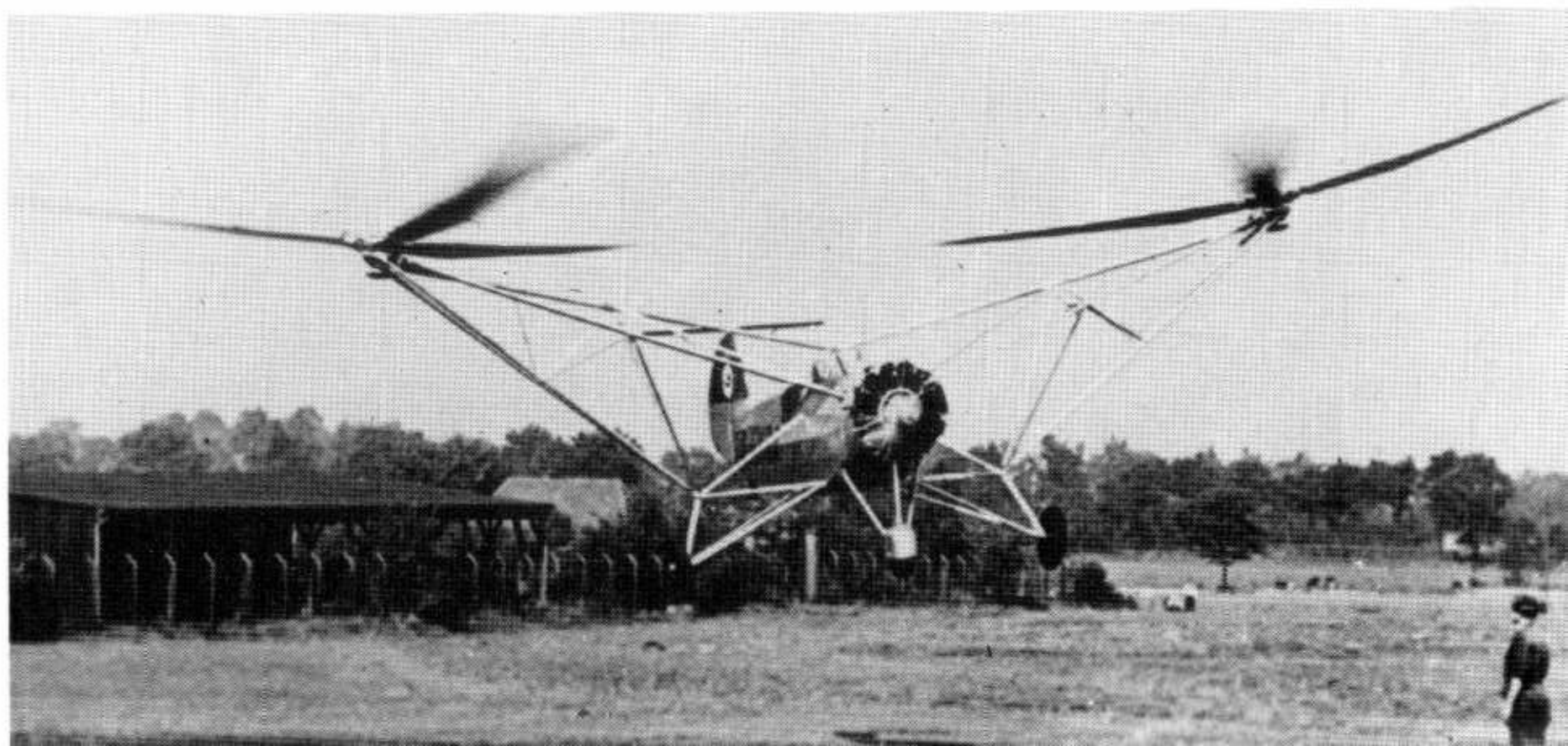
Above: Preparing the Fw 61 V 1, D-EBVU, for takeoff on its first flight. The small airscrew served only to cool the motor. The first flights of the Fw 61 V 1 were made as captive flights.
