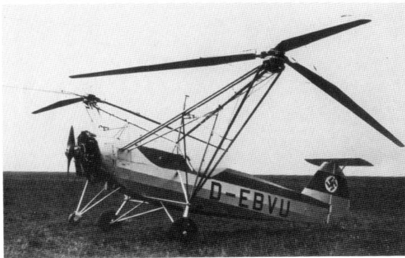
Above: This picture of the Fw 61 shows the design of the rotor carrier especially clearly.
