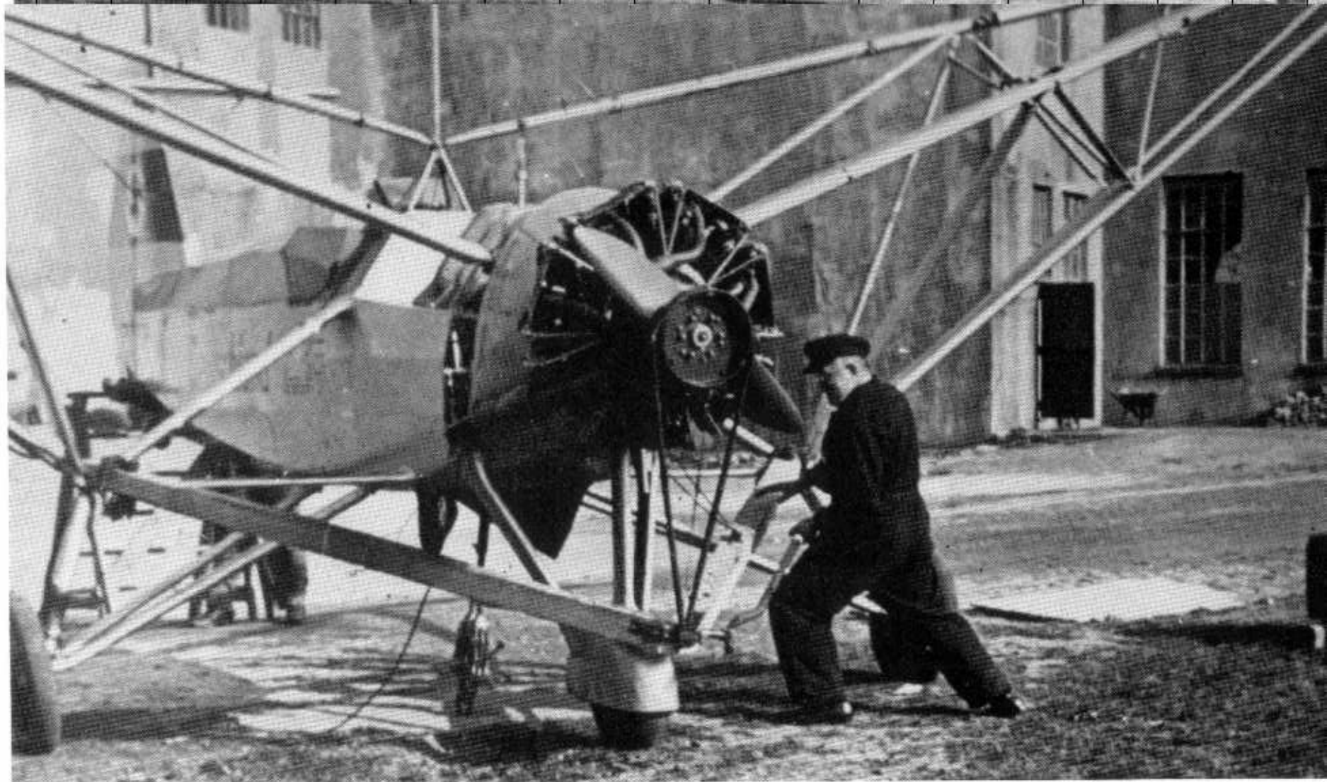
Above: Preparing the Fw 61 V 1, D-EBVU, for takeoff on its first flight. The small airscrew served only to cool the motor. The first flights of the Fw 61 V 1 were made as captive flights.
